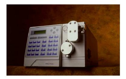
High-performance liquid chromatography (HPLC) also know as high-pressure liquid chromatography is an instrumental system based on chromatography that is widely used in forensic science. The "HP" portion of the acronym is sometimes assigned to the words high pressure (versus high performance), but it refers to the same analytical system. HPLC is used in drug analysis, toxicology, explosives analysis, ink analysis, fibers, and plastics to name a few forensic applications.
